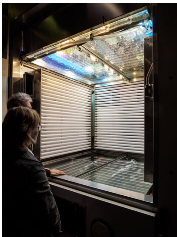
Figure 8.2: View of the sun simulator used in the experiments at EUS.
