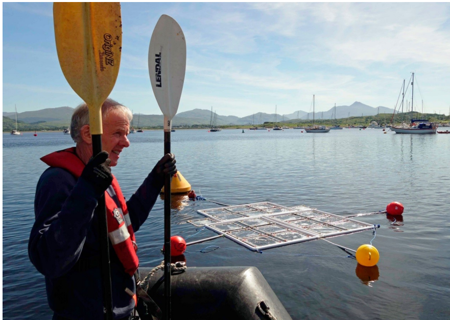
Figure 5.3: Andy McLeod using a range of filtered gas bags to measure photochemical production of dissolved gases in seawater at the ocean surface during the longest day of 2018.
