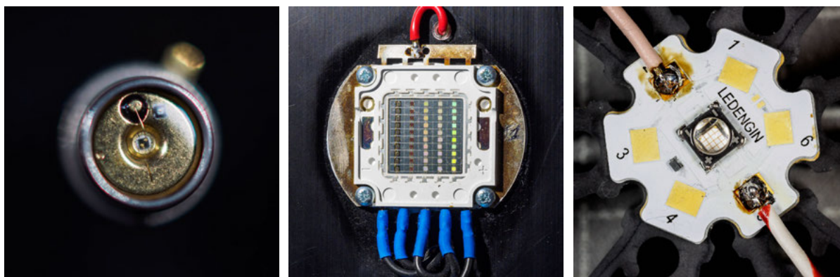
Figure 6.1: Light emitting diodes. a) The first UV LED sold commercially (top view). The LED die can be seen at the center below the flat window (type NSHU550E, Nichia, Japan), b) A custom assembled array with 50 1 W LED dies. This array has five channels, each one with different dies. One of the channels emits at 365 nm. (Shenzhen Weili, Shenzhen, China) c) A 4 W high power LED at 365 nm mounted on a star-board (type LZ1-00UV00 LED Engin, USA).
