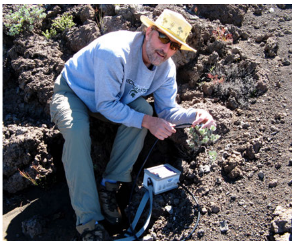
Figure 4.1: Ron Ryel taking epidermal transmittance measurements with a UV-A PAM instrument in 2007.
